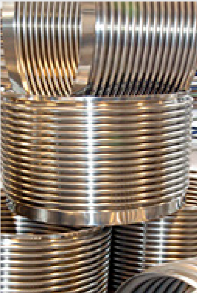
4. The new bellow is made followed by the inner sleeve
