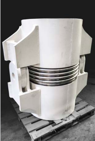
9. Completed Expansion Joint
